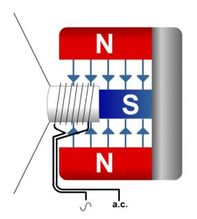
The alternating current that represents a sound wave flows through the coil. As the current carrying coil is inside a magnetic field a force is produced, which makes the coil move. This pulls the paper cone in the same direction. As the current changes direction, the force produced changes direction. This makes the paper cone move the opposite way. The backward and forward motion of the cone produces a sound wave in the air.
