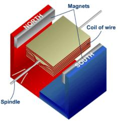
An electric motor uses the motor effect to spin a coil of wire inside a magnetic field.
