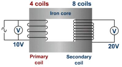
The alternating current in the primary coil has a changing magnetic field around it. This changing field induces an alternating current and voltage in the secondary coil. The size of this voltage depends on the difference in the number of loops on the coils.
