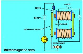
When the small current in the input circuit is switched on, the electromagnet becomes magnetic and attracts the iron armature. The armature rotates towards the electromagnet, pushing the contacts together. This switches on the large current in the output circuit. This type of relay circuit is used in the ignition of a car.
