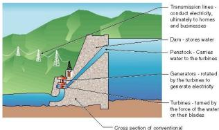
hydropower facility that uses an impoundment dam
