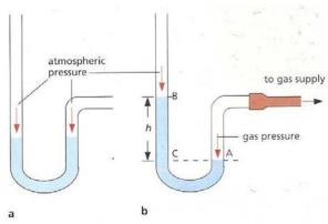
Pressure of gas inside the container in mm Hg = 760mm + difference in mercury height h
