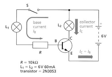
Transistors have many advantages over other electrically operated switches such as relays. They are small, cheap, reliable, have not moving parts, their life is almost indefinite in a well-designed circuit and they can switch on and off millions times a second.
